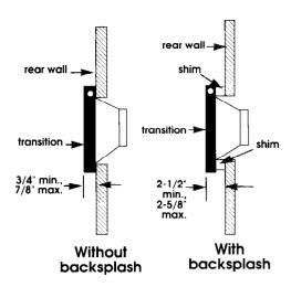
For countertops with a backsplash, the distance from the rear wall to the gasket must be at least 2-1/2"; 2-5/8" maximum.
